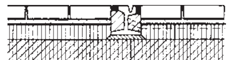
h) Tram track paving with joint sealing pursuant to the Technical Terms of Delivery for Bituminous Joint Sealing Compounds (TLbit Fug)
